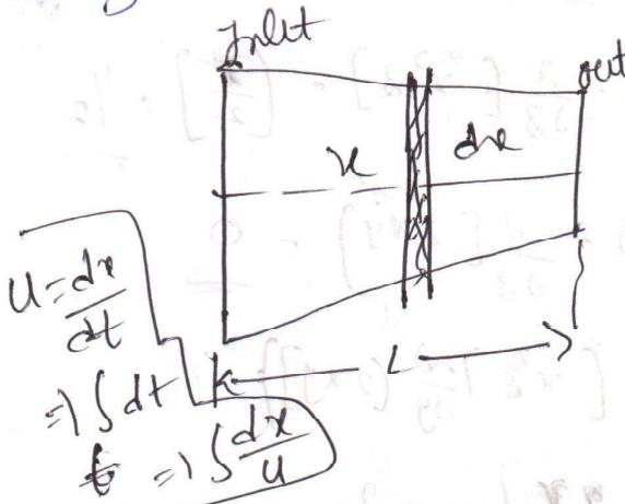
$$\begin{aligned} t &= \int_0^L dt \\ t &= \int_0^L u_0 \left( 1 + \frac{3x}{L} \right)^{\frac{1}{2}} dx \\ &= \frac{1}{u_0} \left[ \frac{1}{3} \log \left( 1 + \frac{3x}{L} \right) \right]_0^L \end{aligned}$$
