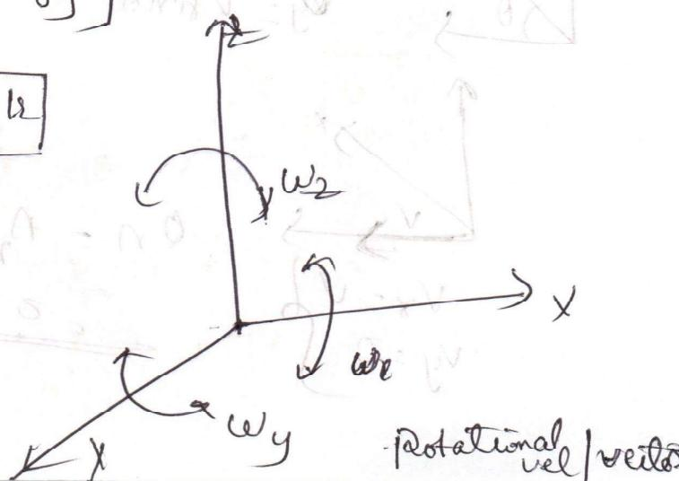
$$\rightarrow \omega_z = \frac{1}{2} \left[ \frac{\partial v}{\partial x} - \frac{\partial u}{\partial y} \right]$$
