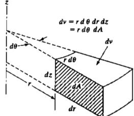
$$\pi = \frac{1}{2} \int_{0}^{2\pi} \int_{A} \sigma^{T} \varepsilon r \, dA \, d\theta - \int_{0}^{2\pi} \int_{A} u^{T} f r \, dA \, d\theta - \int_{0}^{2\pi} \int_{L} u^{T} T r \, dl \, d\theta - \sum_{i} u_{i}^{T} P_{i}$$
