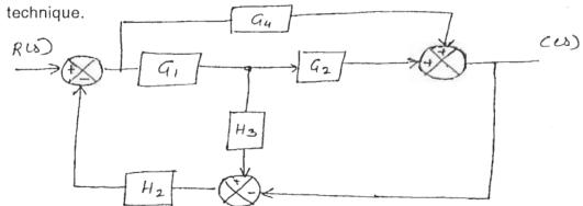
(a) Find the overall transfer function of the system using signal flow graph. 10 3. Using Mason's gain formula.
