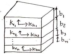
The average permeability kx & ky in the horizontal and ventical direction's one callulated Kx=1/b (Kh, b, + Kh2 b2 + Kh3 b3+ --- Khin bn)
