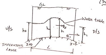
1-> Distance by & Section's (or) waterbodies im-> Maximum head of the water table '-> General Level of the moter table 10-> Level of water body in the ripstream Side 30 -> Discharge towards upstream Side 3, -> Dischange towards downstream side
