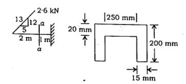
With the help of moment area method, determine the displacement at C for the steel overhanging beam as shown in the figure  $E_{ST} = 200 \, \text{GPa}$ [Assume below.  $I = 50 \times 106 \text{ mm}^4$
