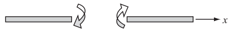
Fig. S2.7 Sign convention: positive bending moment M anticlockwise on a positive face and clockwise on a negative face
