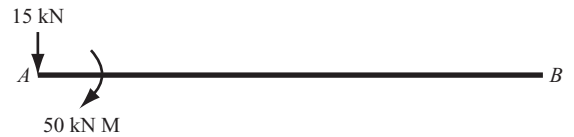
(b) Equivalent force – Moment at A
