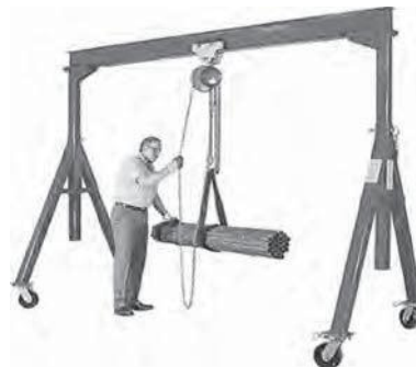
A Hoist Used in a Workshop
