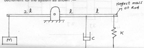
4. (a) Find the Lowest natural frequency of transvrse vibration of system as shown 12 by Raleigh's method.
