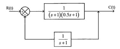
a) Draw the signal flow graph for the following feedback control system.
