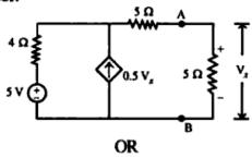
Obtain the Norton's equivalent circuit for the circuit given in figure.
