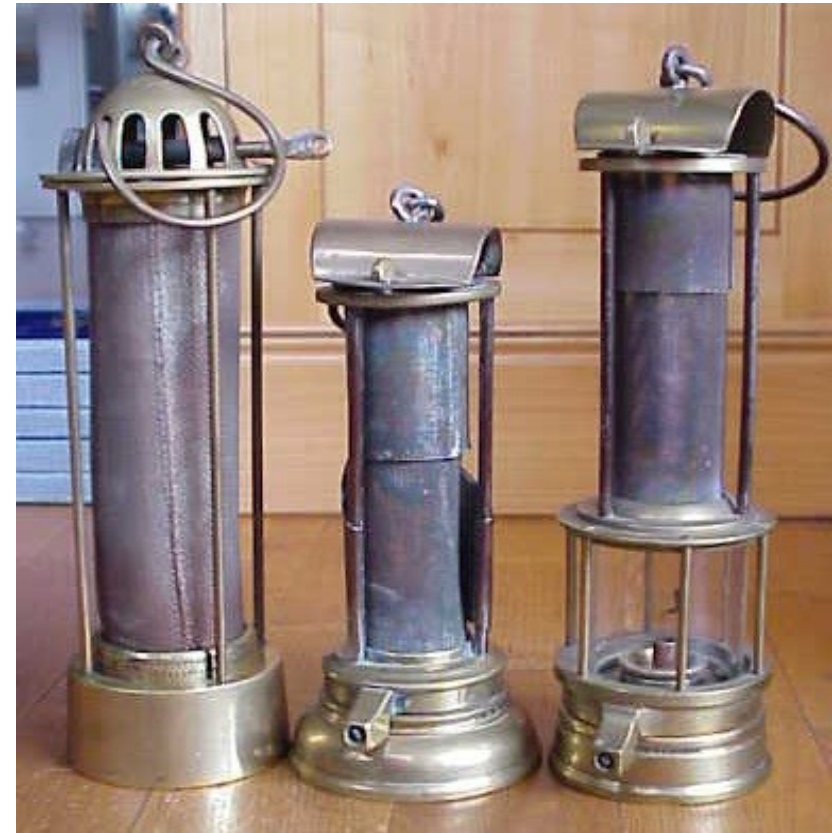
Three early flame safety lamps - From left to right Stephenson , Davy & Clanny Types.
