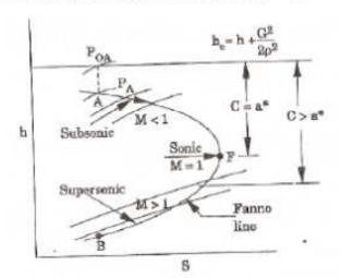
The equation which yields the fanno line for the given values of h<sub>0</sub> and G is called "fanno flow equation".
