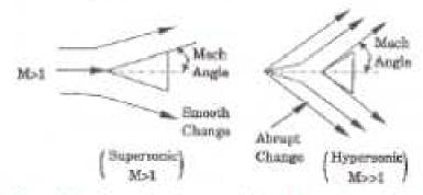
Mach angle is formed, when an object is moving with supersonic speed. The wave propagation and changes are smooth. When an object is moving with hypersonic speed the changes are abrupt is shown in Fig. Hence for a supersonic flow over two – dimensional object "mach wedge" is used instead of "mach cone".
