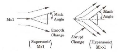
Mach angle is formed, when an object is moving with supersonic speed. The wave propagation and changes are smooth. When an object is moving with hypersonic speed the changes are abrupt is shown in Fig. Hence for a supersonic flow over two – dimensional object "mach wedge" is used instead of "mach cone".
