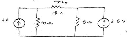
(ii) Determine the Thevenin's equivalent circuit with respect to the terminals a and b for the circuit shown below.
