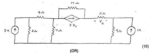
12.b) Determine the nodal voltages for the following circuit
