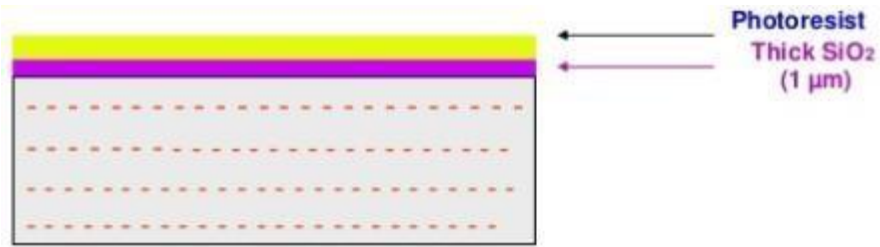
c. Photoresist on the layer of SiO 2
