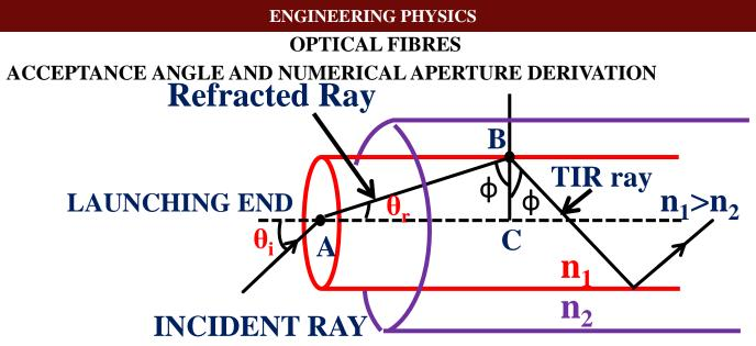
In the optical fibre, core and cladding arrangement is in such a way that the core acts like a parallel mirrors. The message which has to be sent via optical fibre is first being encoded into light wave and fed into the fibre as shown in the figure. Multiple internal reflections within the core results in propagation of light within the core.
