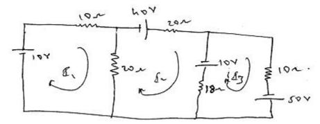
For the circuit shown above find  $I_1$ ,  $I_2$  and  $I_3$  using loop-current method. (5)
