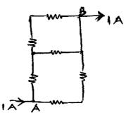
5. Find the value of load resistance  $(R_L)$  for which the power source will supply maximum power. Also find the value of the maximum power for the network as shown below :
