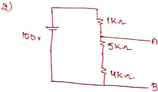
Voltage drop AB is  $V_{AB} = 100 \times \frac{5+4}{1+5+4} = 90\text{V}$
