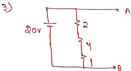
Voltage drop AB is  $V_{AB} = 20 \times \frac{2+4+1}{2+4+1} = 20 \times \frac{7}{7} = 20\text{V}$
