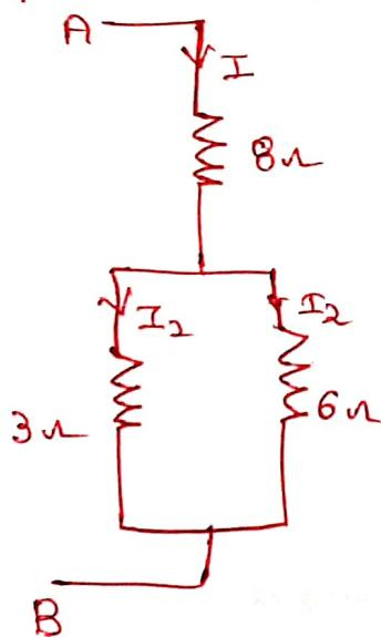
$$3 \& 6 \text{ are in parallel} = (3 \parallel 6) = \frac{3 \times 6}{3+6} = 2\Omega$$
