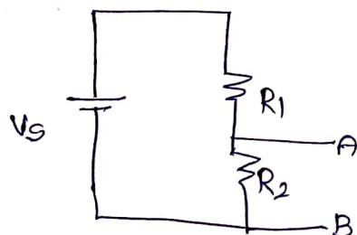
$$V_{AB} = V_S \times \frac{R_2}{R_1 + R_2}$$
