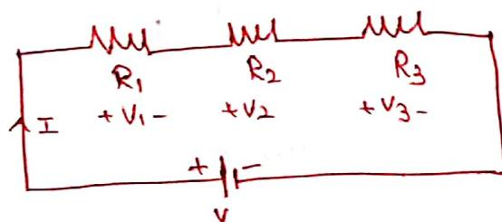
The Resistances  $R_1$ ,  $R_2$  &  $R_3$  are connected in series
