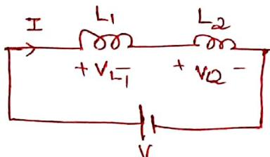
$$V = V_{L1} + V_{L2}$$
