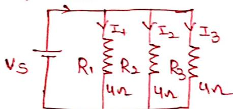
$$I_1 = I_T \times \frac{(R_2 \parallel R_3)}{R_1 + R_2 + R_3} \Rightarrow 12 \times \frac{\left(\frac{4 \times 4}{4+4}\right)}{4+2} = 4A$$
