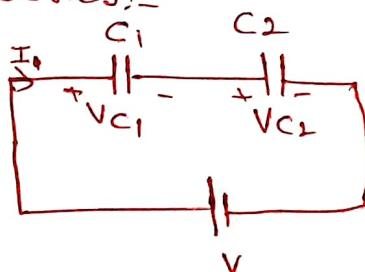
$$V = V_{C_1} + V_{C_2}$$
