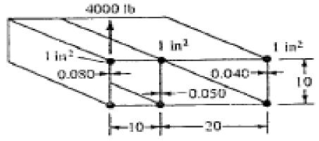
3. Find the internal loads acting on each member of the shown in fig.
