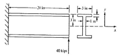
5.a) Find the bending stress at any points A, B and of the beam cross – section shown in figure below.
