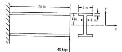
3.a) Find the bending stress at any points A, B and of the beam cross – section shown in figure below.
