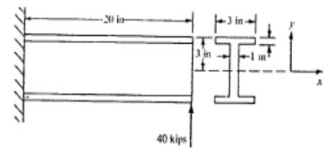
7.a) Find the bending stress at any points A, B and of the beam cross – section shown in figure below.
