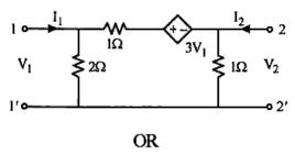
Determine the driving point impedance of the network given below.
