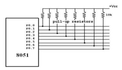
(A pull-up resistor weakly "pulls" the voltage of the wire it is connected to towards its voltage source level when the other components on the line are inactive.)
