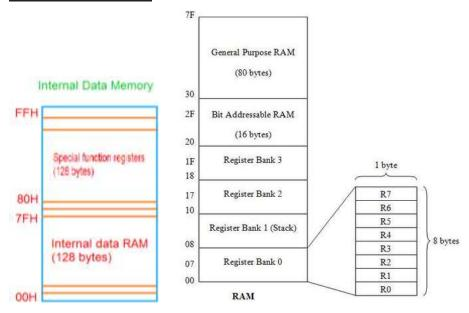
The internal data memory consists of 256 bytes, these are divided into two parts:
