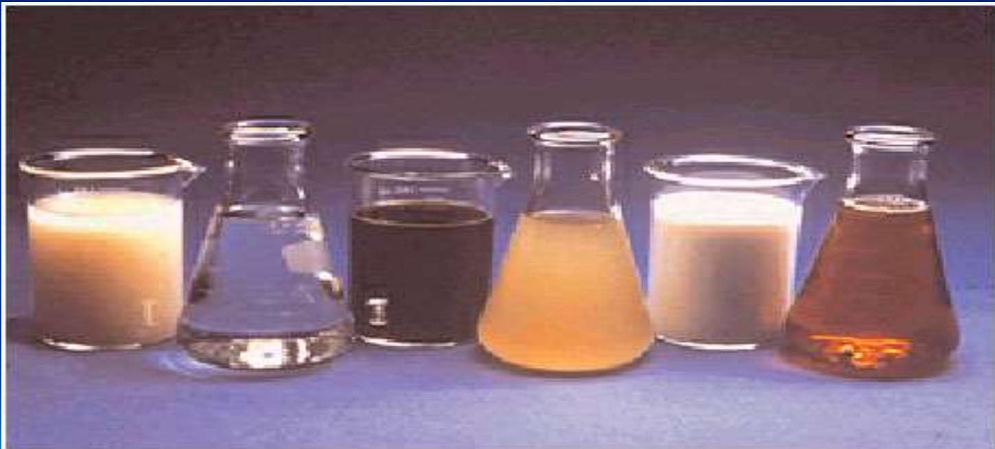
Fig. 6-1. Liquid admixtures, from left to right: antiwashout admixture, shrinkage reducer, water reducer, foaming agent, corrosion inhibitor, and air-entraining admixture. (69795)
