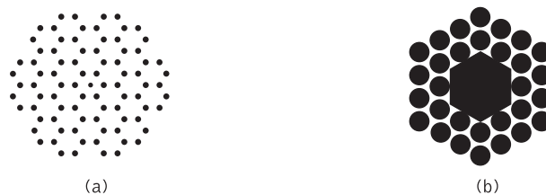
Figure 2.38 Photonic bandgap (PBG) fiber structures in which the dark areas are air (lower refractive index) and the lighter area is the higher refractive index: (a) honeycomb PBG fiber; (b) air-guiding PBG fiber
