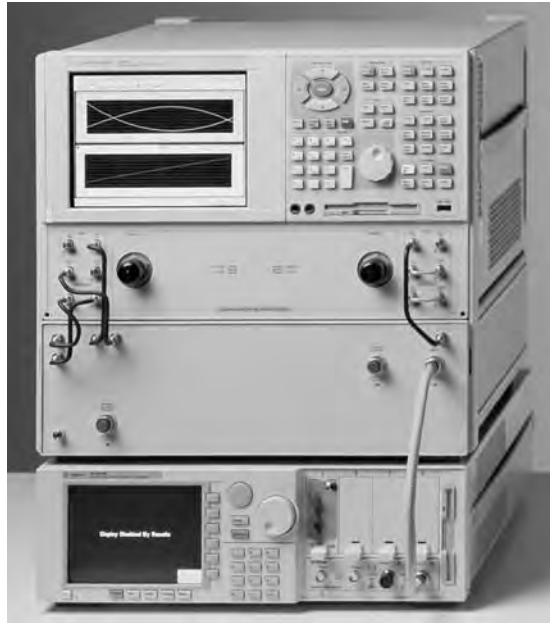
Figure 14.12 Optical fiber dispersion measurement and analyzer [Ref. 33]. © Agilent Technologies, Inc. 2005. Reproduced with permission, courtesy of Agilent Technologies, Inc.
