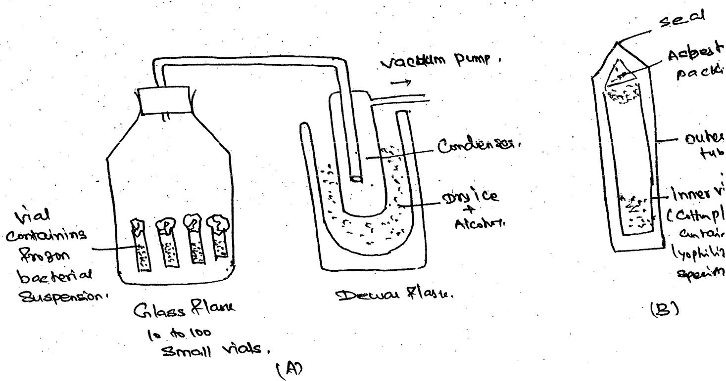
(A) small cotton-plugged vials containing frozen Suspension of the m/s are placed in the glass-flask, which is attached to a condenser;
