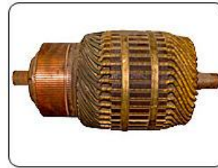
Armature with steel binding wire
