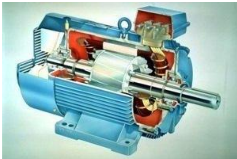
Fig. 8 Cut sectional view of the induction motor.
