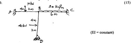
VIII. Analyse the frame shown in the figure by moment distribution method. Draw BMD. (15)
