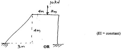
IX. Analyse the beam shown in the figure by moment distribution method. Draw BMD and SFD.
