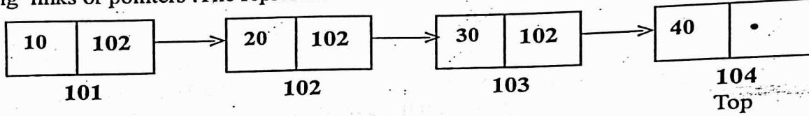
In the above stack contains four nodes like 10, 20, 30and 40. Here the 40 is top node because it is most recently element. Manipulate the linked stack by using 3 types of operations like.
