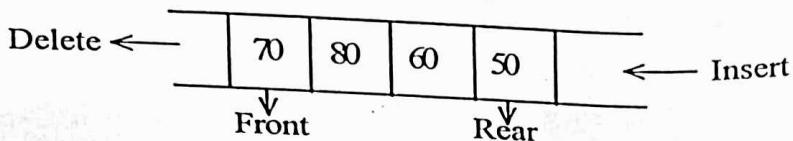
INSERT: Before inserting an element in to the queue we have to check the condition whether it is full or not. for this , the condition is if MAX=REAR then we will say the QUEUE is full Otherwise increment REAR by one & push that element into Q[rear].
