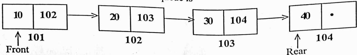
In the above queue contains 4 elements like 10, 20, 30 and 40. On that 10 is FRONT node and 40 is REAR node. To develop the linked queue by using 3 types of operations like
