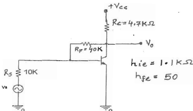
6. (a) Determine the lower cutoff frequency for the following network.
